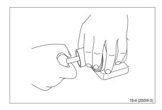
(14) Draw the inner and outer parts of the assembly tool out of the steering unit bore, leaving the guide from the inner part in the bore.
