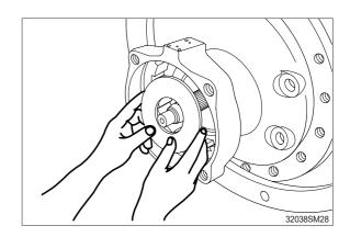
(6) Insert the ball guide (11) into the cylinder (9).
