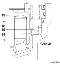
1 Housing 15 Separate plate 9 Cylinder block 16 Brake piston 14 Friction plate 19 Spring
