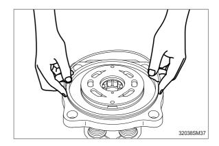
(15) Connect the rear cover (20) with the body (1) and tighten the wrench bolt (24).
