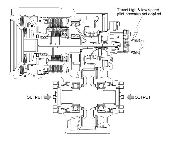
When the travel high/low speed pilot pressure is not applied in the piston space, the piston compress against the multi disk pack due to the spring force. Thus the parking brake is engaged.
