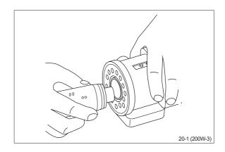
(16) The spool set will push out the assembly tool guide. The O-ring is now in position.
