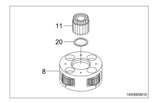
(7) Remove carrier 2 (8) assembly from casing (1).
