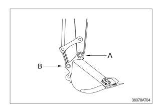
② Remove nut (1), bolt (2) and draw out the pin (B).
