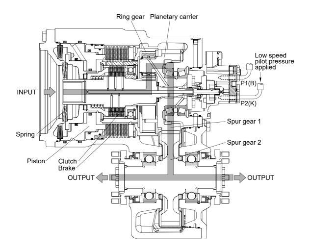
In low speed operation, the internal gear of the planetary drive is backing upon the closed, case-rigid brake. In this speed the piston chamber of the brake is unpressurized, so that the elastic force and additionally the hydraulic pressure of the clutch piston is acting upon the disk pack. At this time the clutch is open, i.e. the hydraulic released.
