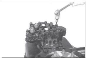
14) Loosen cover screws, remove cover and gasket (see also 14WF8TM286).
