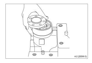
(3) Lift the gearwheel set (with spacer if fitted) off the unit. Take out the two O-rings.
