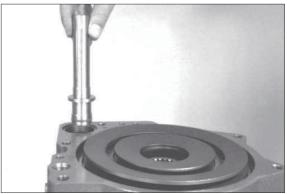
61) Place O-ring (see arrow) into annular groove of housing and insert compression spring.
