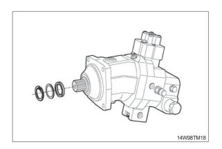
(1) Protecting the drive shaft. Remove retaining ring and shim.
