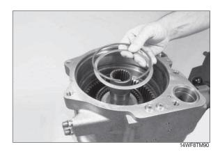
27) Take disk package of clutch with end plate(s) out of ring gear.
