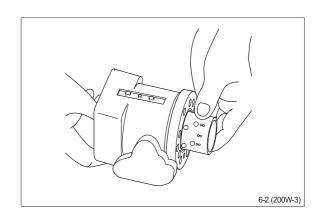
(10) Take ring, bearing races and needle bearing from sleeve and spool. The outer(thin) bearing race can sometimes "stick" in the housing, therefore check that it has come out.
