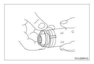
(8) Fit the cross pin into the spool / sleeve.
