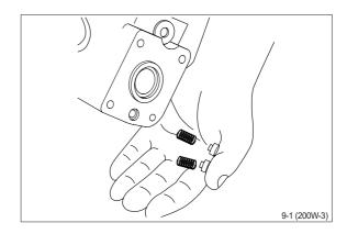
⑤ The dual shock valves are now disassembled.
