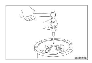
(15)Remove the needle bearing (21) from the rear cover (20) by using slide hammer bearing puller.
