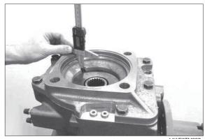
38) Determine Dim. C (Measuring hole II) from mounting face/housing to front face/piston (brake).
