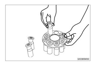
(8) Reassemble the piston assembly (9) to the body (1).
