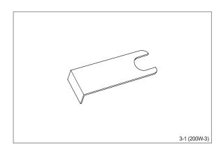
(4) Assembly tool for dust seal (1).
