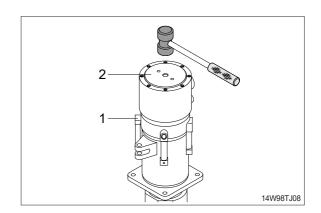
(4) Fit shim (12), and spacer (4) to hub (1) of turning joint upside.
