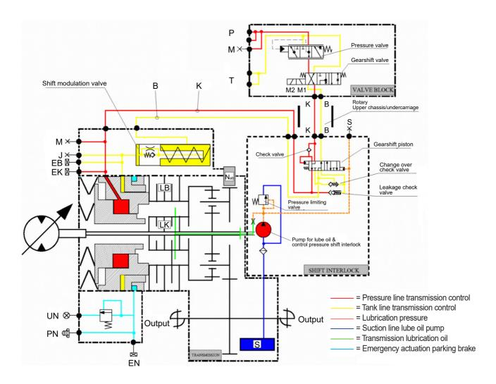
Measuring points-Transmission/Shift interlock:
