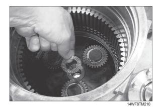
23) Insert preassembled input shaft (with ring gear).
