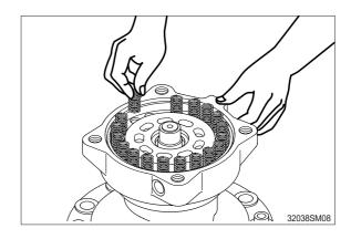
(9) Remove brake piston (16) from body (1).
