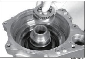
20) Remove pressure piece and compression spring.
