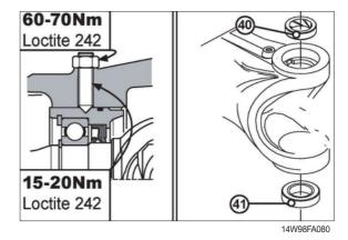
(7) Screw the check nuts of the dowels and lock them using a dynamometric wrench.
