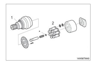
Remove fixing screw (cylinder).
