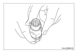
(4) Guide the spool into the sleeve. Make sure that spool and sleeve are placed correctly in relation to each other.
