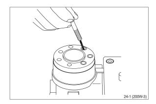
(31) Fit the six screws with washers and insert them. Cross-tighten all the screws and the rolled pin.
