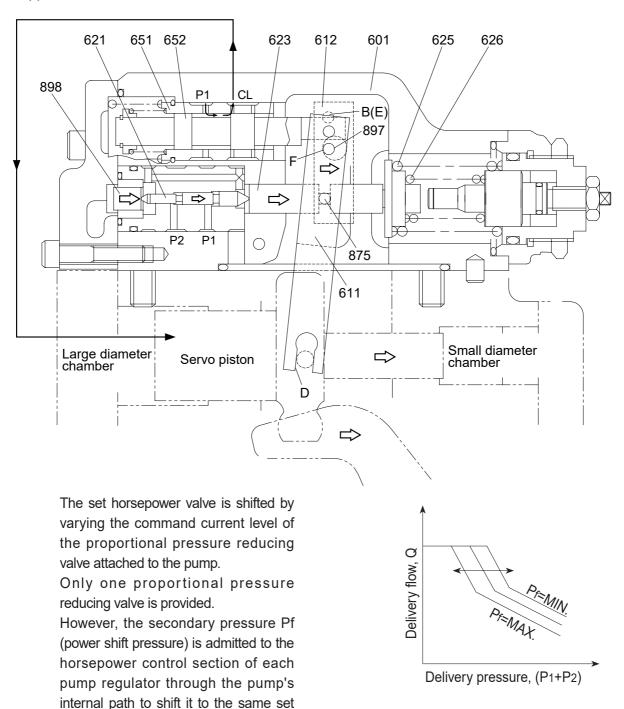
This function permits arbitrary setting of the pump output power, thereby providing the optimum power level according to the operating condition.
