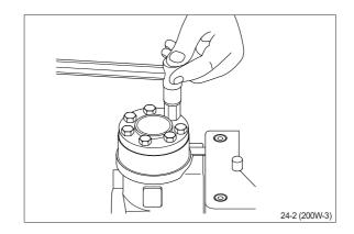
(32) Place the dust seal ring in the housing.
