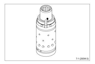
(12) Carefully press the spool out of the sleeve.
