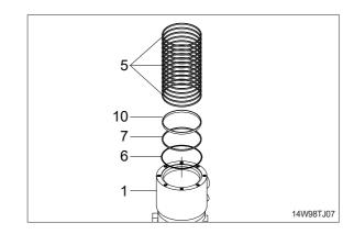
(3) Set shaft (2) on block, tap hub (1) with a plastic hammer to install.
