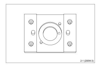
(2) Assembly tool for O-ring (5,13,16) and kin-ring (6).
