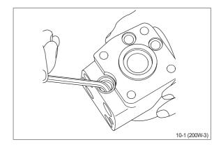
③ Shake out spring and piston. The valve seat is bonded into the housing and cannot be removed.
