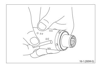
(9) Fit bearing races and needle bearing as shown on below drawing.
