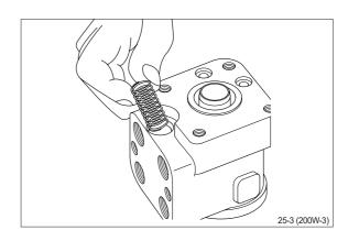
(37) Screw in the setting screw with an 8mm hexagon socket spanner. Make the pressure setting on a panel or the machine.
