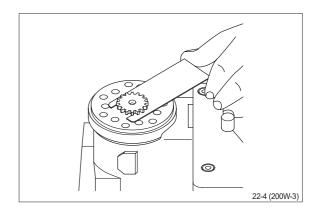
(26) Grease the two O-rings with mineral oil approx. viscosity 500 cST at 20°C and place them in the two grooves in the gear rim. Fit the gearwheel and rim on the cardan shaft.
