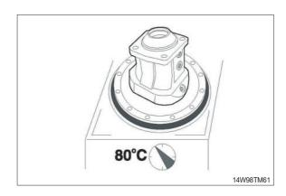
(4) Insert rotary group into housing to seat position.
