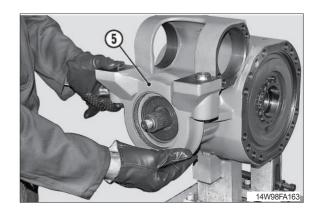
(6) Remove the sealing ring (6).
