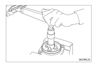
(12) Assemble swash plate (20) to joint (19).
