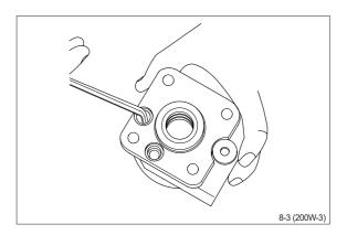
④ Shake out the two springs and two valve balls into your hand. The valve seats are bonded into the housing and cannot be removed.
