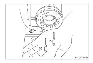
(9) Take care to keep the cross pin in the sleeve and spool horizontal. The pin can be seen through the open end of the spool. Press the spool inwards and the sleeve, ring, bearing races and needle bearing will be pushed out of the housing together.
