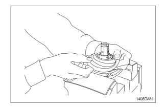
(15) Fit boot (26) and lock nut (22), and handle subassembly is assembled completely.
