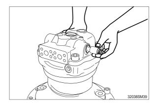
(17) Insert O-rings to the relief valve (30) and reassemble them to rear cover (20).
