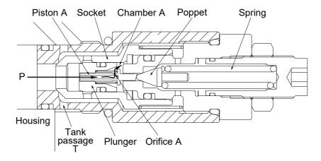
(2) When the pressure at port P becomes equal to the set pressure of the spring, the pressurized oil pushes open the poppet and flows to tank passage (T) through the plunger internal passage, orifice A, chamber A, periphery orifice B and hole E.
