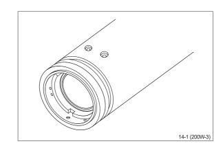
(2) Place the two flat neutral position springs in the slot.
