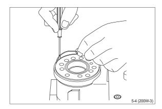
(8) Shake out the check valve ball and suction valve pins and balls.
