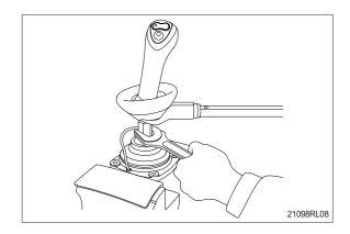
(19) Apply grease to rotating section of joint and contacting faces of disk and push rod.
