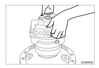
(16)Insert check (29) and spring (28) in the valve casing and install O-ring (27) and back up ring (26). Tighten plug (25) to the rear cover (20).
