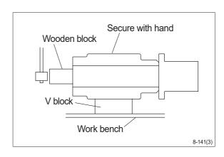
(5) Remove seventeen slipper seal (5), O-ring (6, 7) and wear ring (10) from hub (1).
