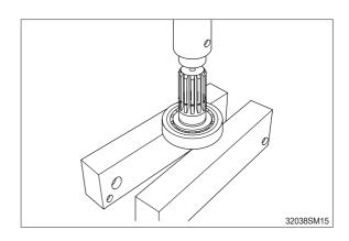
(14)Remove bushing (6) and oil seal (2) from body (1).
