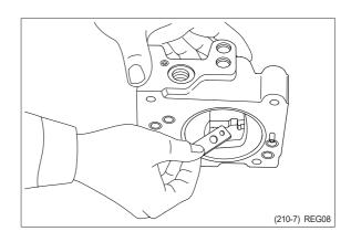
(10) Draw out pin (874) and remove feedback lever (611).
