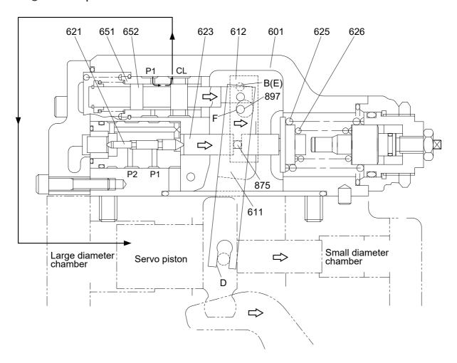
When the self pump delivery pressure P1 or the companion pump delivery pressure P2 rises, it acts on the stepped part of the compensating piston (621). It presses the compensating rod (623) to the right till the force of the outer spring (625) and inner spring (626) balances with the hydraulic force. The movement of the compensating rod is transmitted to lever 1 (612) via pin (875).
