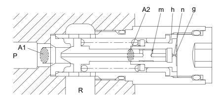
$\@Displayskip$  When hydraulic oil pressure (P $\times$ A1) reaches the preset force (FsP) of spring (4), the plunger (3) moves to the right as shown.
