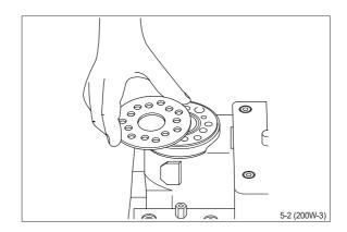
(6) Screw out the threaded bushing over the check valve.
