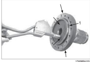
(2) Mount preassembled hub carrier to the axle housing, considering the installation position, and fix it with hexagon screws.
