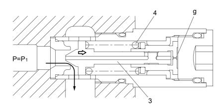
③ The oil flow chamber g via orifice m and n. When the pressure of chamber g reaches the preset force (FSP) of spring (4), the piston (6) moves left and stop the piston (6) hits the bottom of bushing (7).
