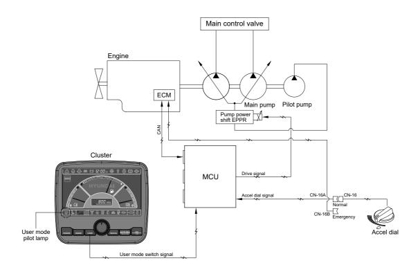
1) High idle rpm, auto idle rpm and EPPR pressure can be adjusted and memorized in the U-mode.
