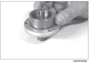
Position ball – (see arrow, engagement for inner rotor) with grease into countersink of pump shaft.
