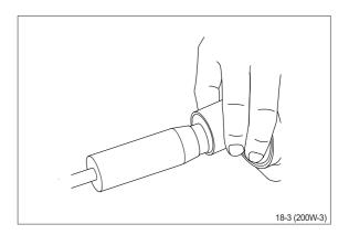
(13) Press and turn the O-ring into position in the housing.
