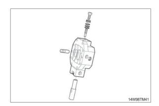
(1) Loosen fixing screw.
