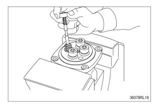
(5) Assemble O-ring (15) onto plug (14).
