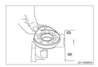
(23) Place the distributor plate so that the channel holes match the holes in the housing.
