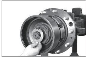
(18) Mount thrust washer with shoulder showing to the retaining ring (outwards).
