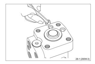
(42) Screw plug with seal ring into the two shock valves using a 6mm hexagon socket spanner.
