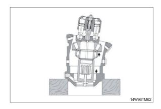
(5) Insert rotary group into housing to seat position.
