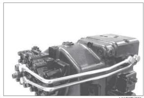
13)Loosen threaded joint of shift interlock (3 x cylindrical screws) and remove cpl. shift interlock.
