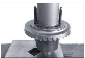
(12) Fix differential with press and tighten crown wheel with cylindrical screws.
