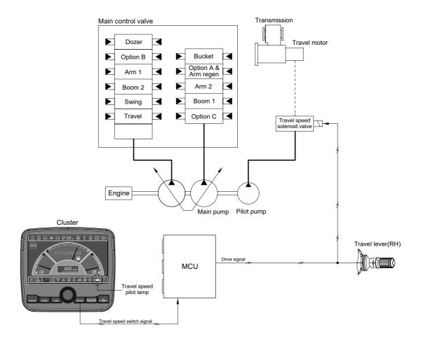
Travel speed can be switched manually by turning the travel speed switch on the RH multifunction switch.
