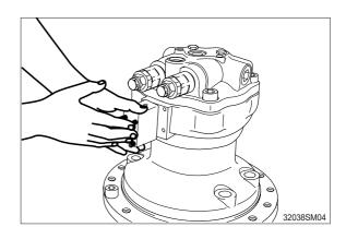
(5) Remove the relief valve (30) from rear cover (20).
