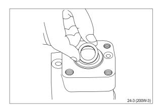
(33) Fit the dust seal ring in the housing.
