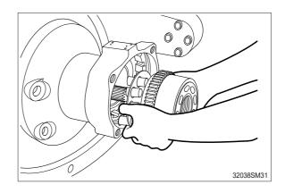
(9) Assembly friction plate (14) and separate plate (15) to the body (1).
