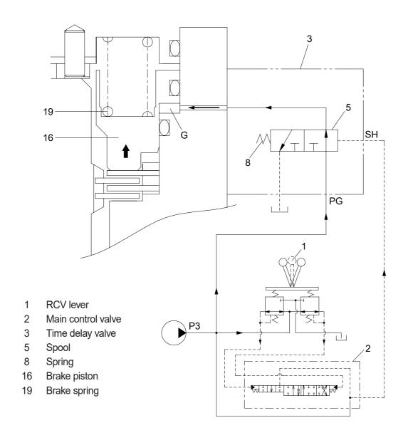
b. When all of the RCV lever (1) are set the neutral position, the spool (5) returns to right. Then, the piston (16) is moved lower by spring force and the return oil from the chamber G flows back to tank port.
