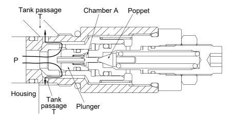
(4) The pressure at port P becomes lower than set pressure of the spring, the poppet is seated by spring force. Then the pressure at port P becomes equal to set pressure of the spring and the plunger is seated to the socket.
