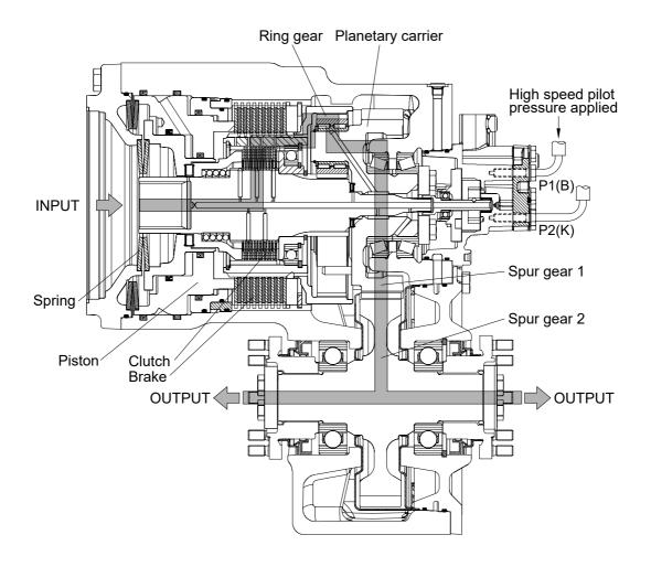
In high speed operation, the clutch is held closed under spring pressure and the brake is hydraulically opened.
