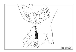
④ The pressure relief valve is now disassembled.
