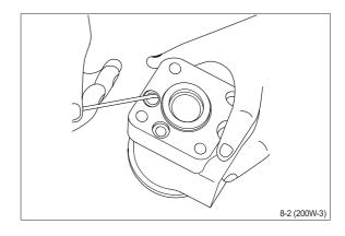
③ Unscrew the setting screws using a 6 mm hexagon socket spanner.
