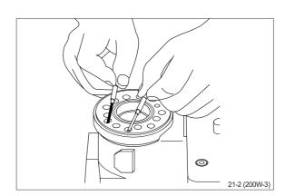
(21) In some cases a spring has to be fitted on the pin before it is placed in the housing.
