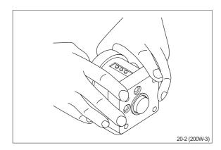
(17) Turn the steering unit until the bore is vertical again. Put the check valve ball into the hole indicated by the arrow.
