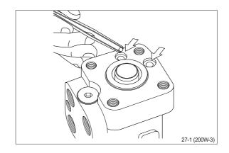
(40) Place springs and valve cones over the two balls.
