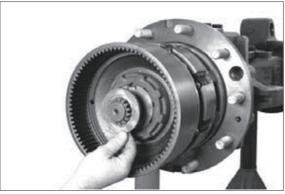
(19) Fix thrust washers by using a retaining ring.
